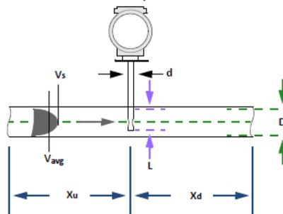
**Image 4.** Installation of Insertion Meters (representative)
