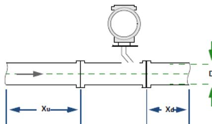
**Image 5.** Installation of In-line Meters (representative)
